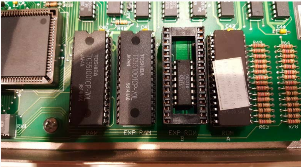
Picture: AVOS circuit board with socketed EPROM chip containing election software. Software upgrades to this machine are installed by physically replacing the chip; as the chip is socketed, this can be done in a matter of seconds. The chip inside a socket is a SmartWatch CMOS real time clock with an NVRAM controller circuit and an embedded lithium energy source.
