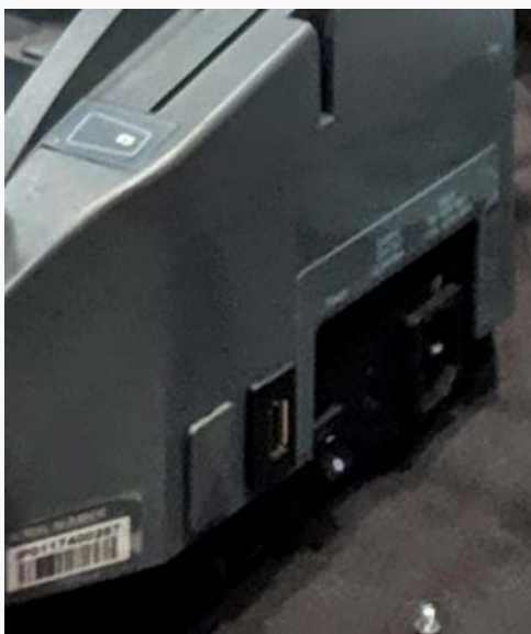
Picture: Externally exposed USB port on the side of the Electronic Pollbook Stand. The port does not get locked when the stand is locked and it does not have a lid or hook on which to place a seal.
